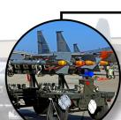
The MHU-141/M munitions trailer is a nuclear certified, four-wheeled automotive steering vehicle capable of ransporting loads of up to 5,700 pounds.
